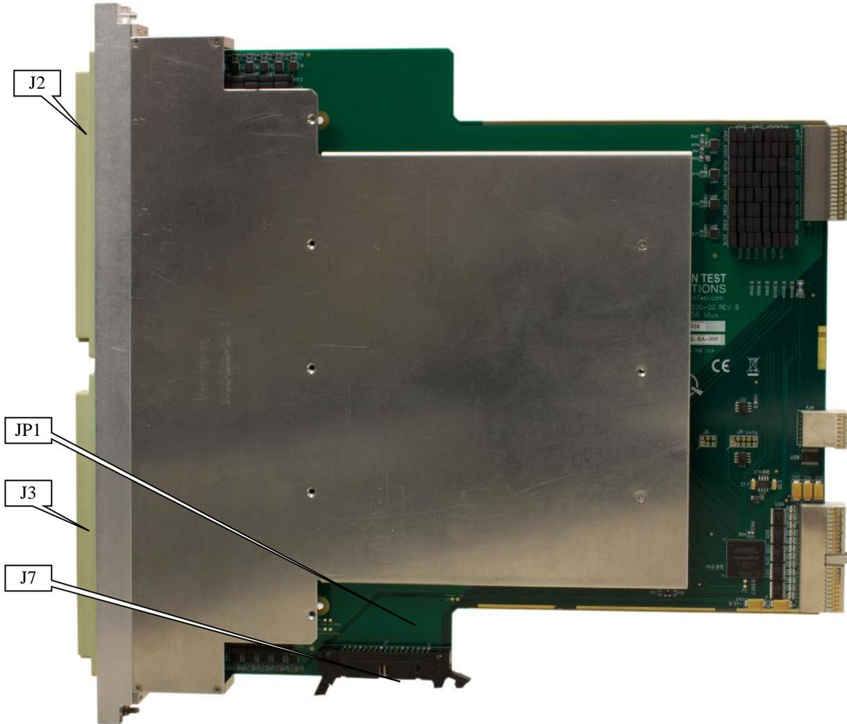
**Figure 3-4: GX6256 Connectors and Jumpers**
