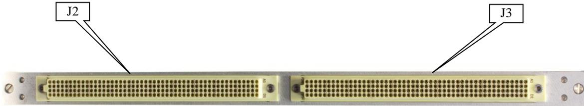
Figure 3-7: GX6256 front Connectors
