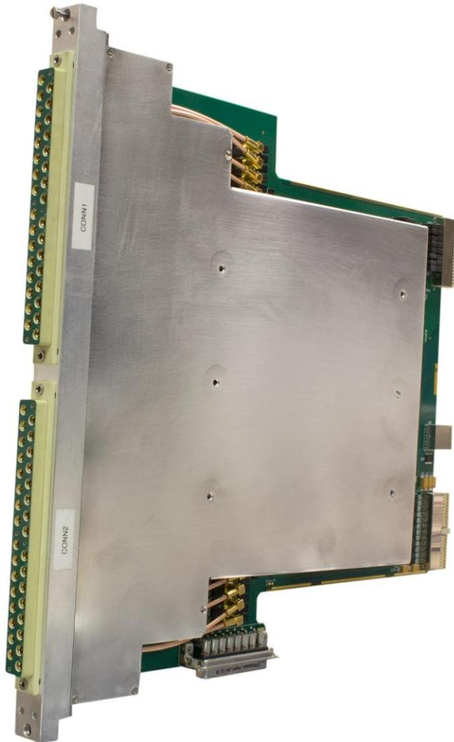
**Figure 2-4: GX6864 Video Multiplexer board**
