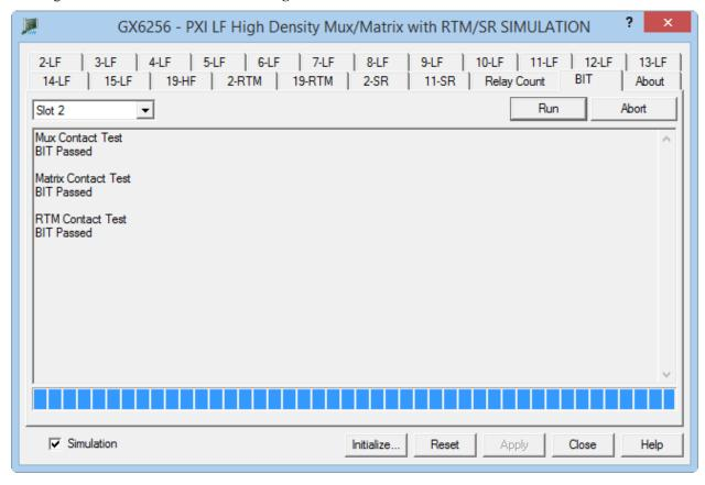
Figure 2-24: Virtual Panel - Built In Test (BIT) Page
