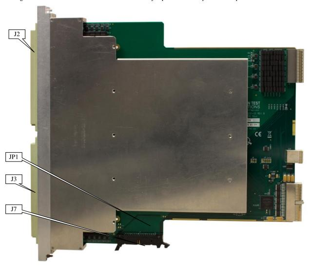
Figure 3-4: GX6256 Connectors and Jumpers
