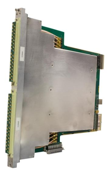
Figure 2-4: GX6864 Video Multiplexer board
