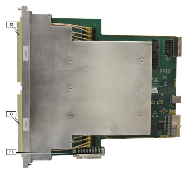
Figure 3-6: GX6864 Connectors and Jumpers
