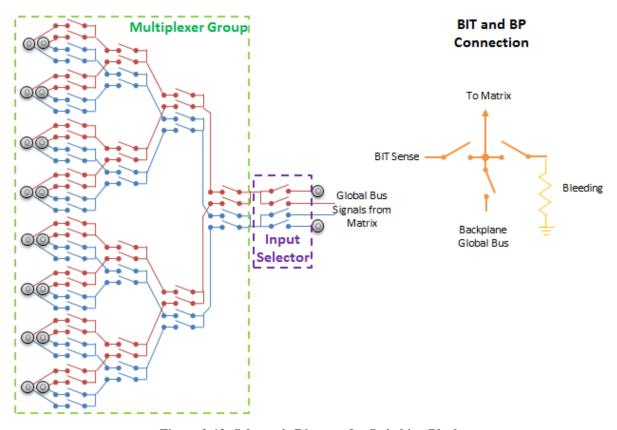
Figure 2-13: Schematic Diagram for Switching Blocks
