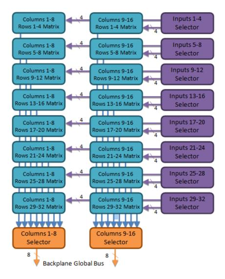
Figure 2-14: Block Diagram of the Switching Sections of the RTM
