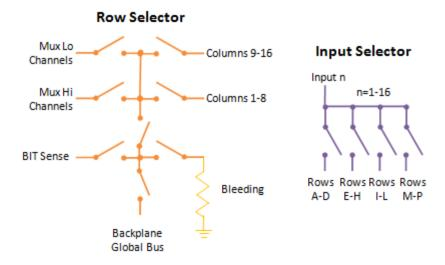
Figure 2-11: Schematic Diagram for Selectors
