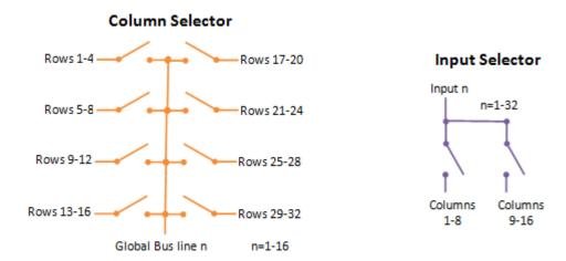
**Figure 2-15: Schematic Diagram for RTM Selectors**
