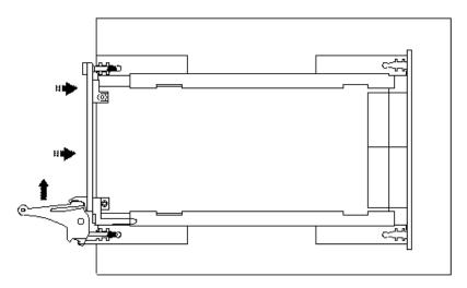
Figure 3-3: Ejector handles position after module insertion
