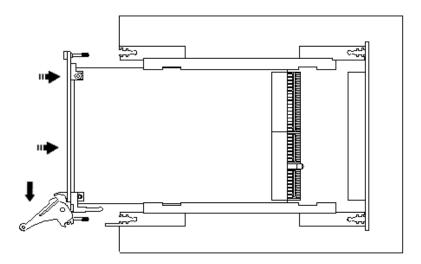
Figure 3-2: Ejector handles position during module insertion
