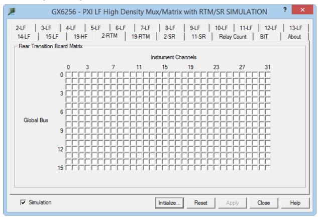
Figure 2-21: Virtual Panel - Rear Transition Module (GX6032) Page
