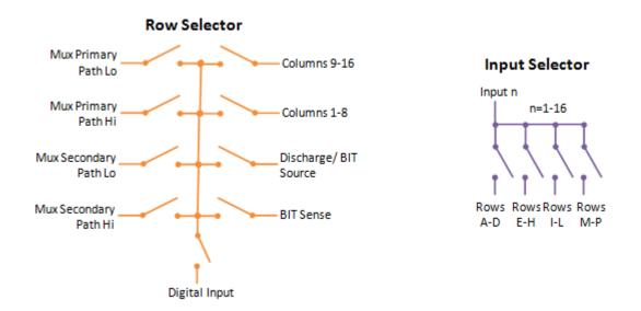
Figure 2-9: Schematic Diagram for Selectors
