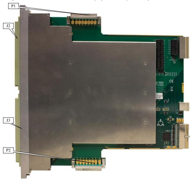
Figure 3-5: GX6192 Connectors and Jumpers
