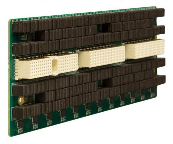
Figure 2-6: GX6009 Switch Router (SR)
