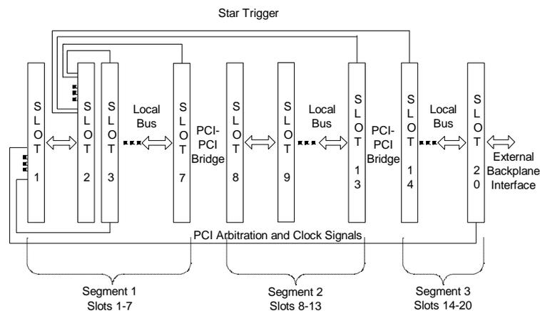
**Figure 2-13: PXI Local Bus Routing**
