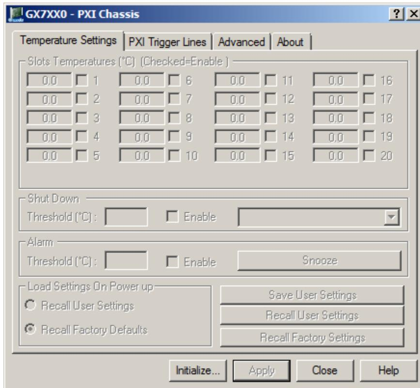
Figure 2-15: GxChassis Virtual Panel – Temperature Settings (not Initialized)
