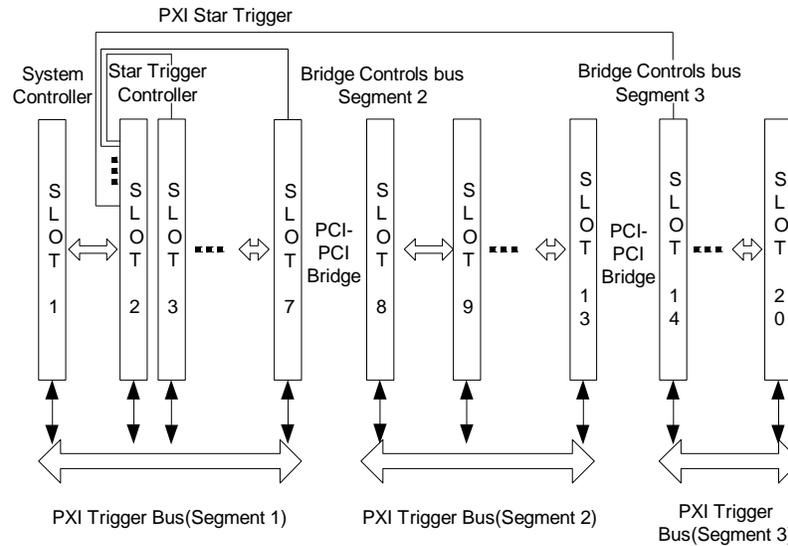
**Figure 2-14: PXI Trigger Architecture**
