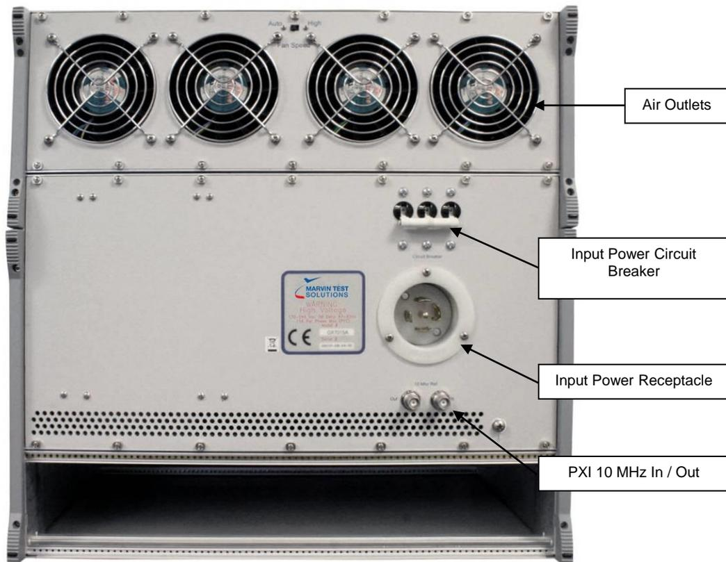
**Figure 2-10: GX7015A/C Rear View**
