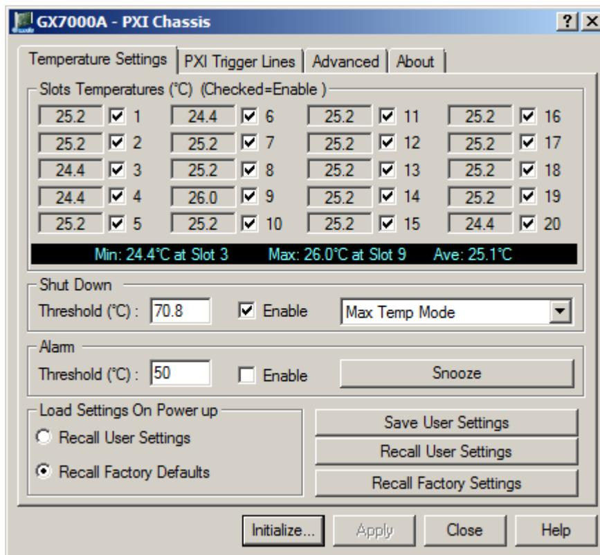
Figure 2-17: GxChassis Virtual Panel – Temperature Settings
