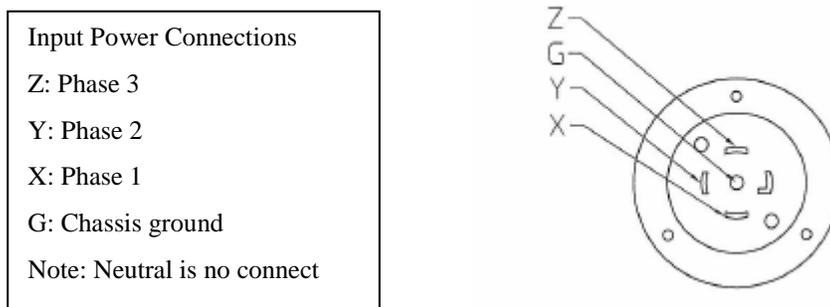
**Figure 3-1: Input Power Connector (Rear Panel View)**
