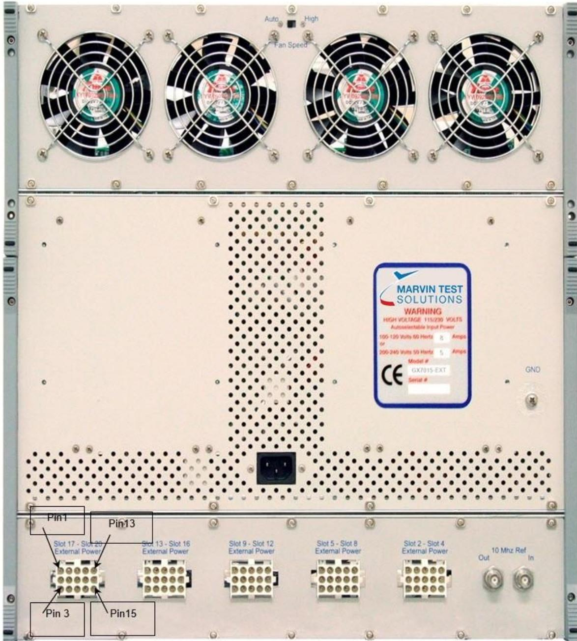
Figure D-1: GX7015-EXT, Rear Panel; Power Connections
