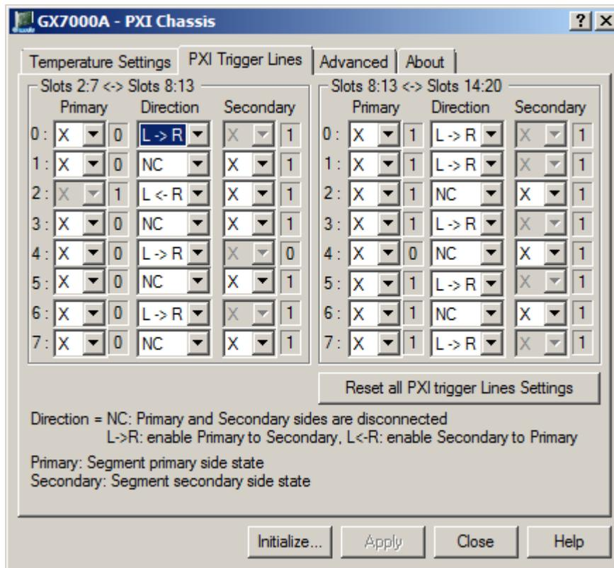
**Figure 2-18: GxChassis Virtual Panel – PXI Trigger Lines**
