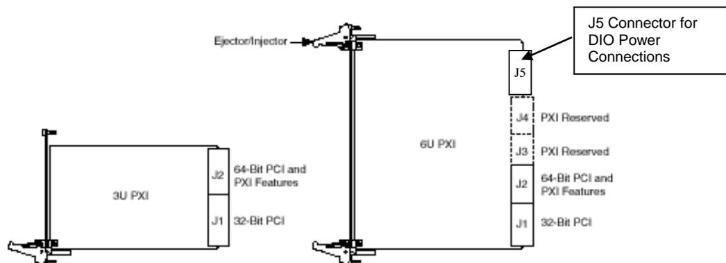
Figure 2-12: 3U and 6U PXI Boards
