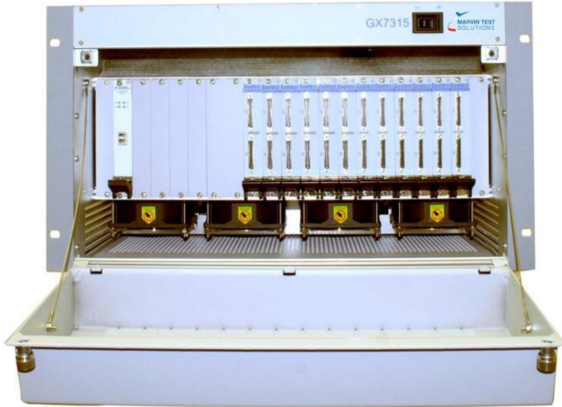
Figure 2-4: GX7315 Front View with Cards Installed, Front Panel Down
