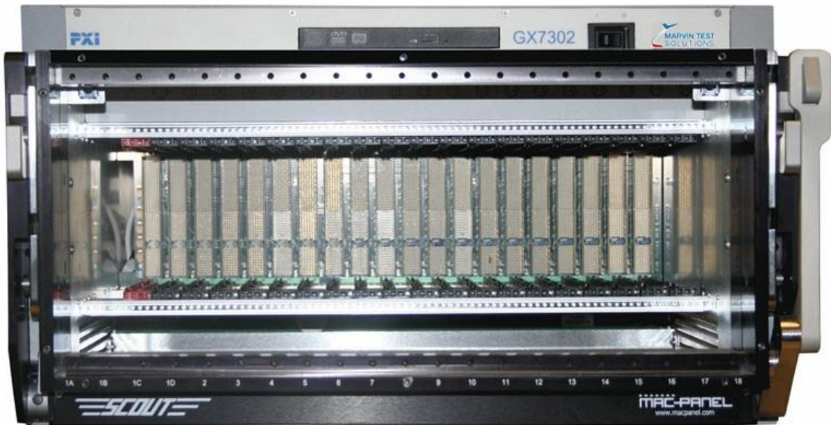
Figure 2-2: GX7302 Front View with a Left Panel Removed
