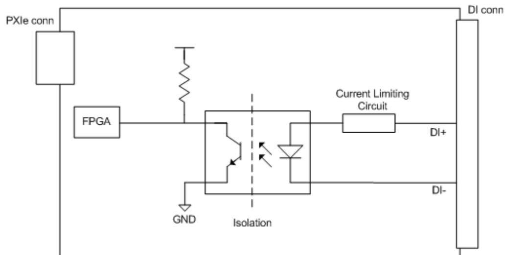
FIGURE 2-16: EMX-7515 BLOCK DIAGRAM
