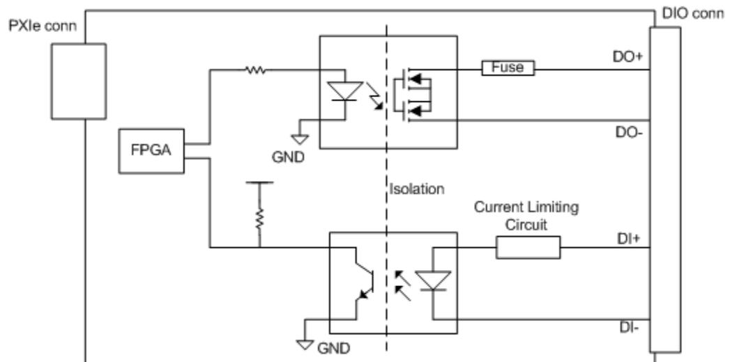
FIGURE 2-12: EMX-7513 BLOCK DIAGRAM
