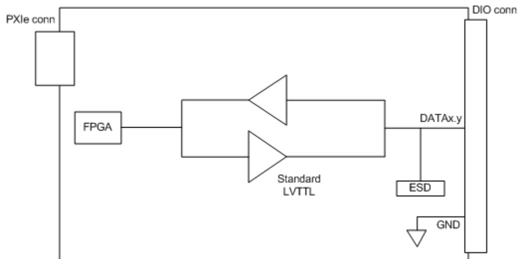
FIGURE 2-10: EMX-7512 BLOCK DIAGRAM
