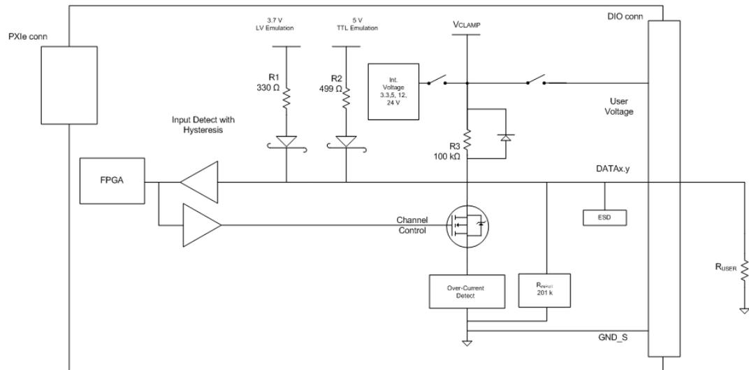
**FIGURE 2-5: TTL/LV EMULATION SOURCING CURRENT TYPICAL CONNECTION**
