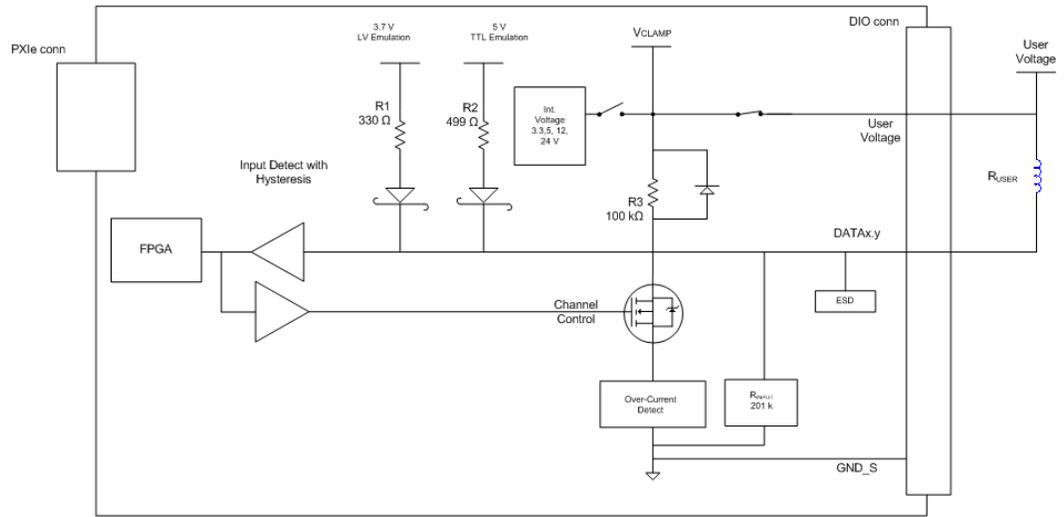
**FIGURE 2-6: SINKING CURRENT TYPICAL CONNECTION**
