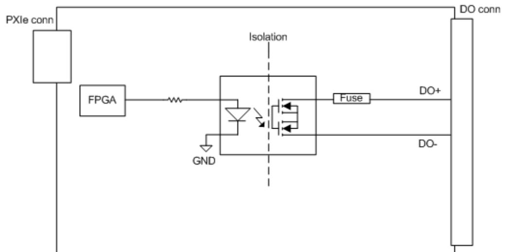
FIGURE 2-14: EMX-7514 BLOCK DIAGRAM
