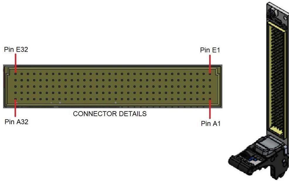
**FIGURE 2-3: EMX-7510 FRONT PANEL DETAIL**
