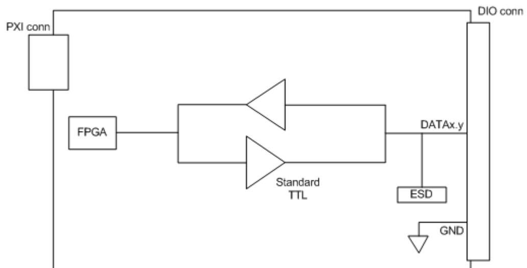
FIGURE 2-8: EMX-7511 BLOCK DIAGRAM
